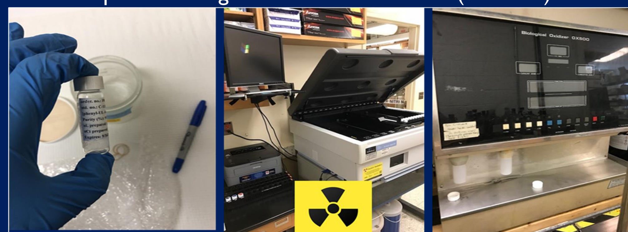
Figure 2a. 14 C-simazine solution Figure 2b. Liquid Scintillation Analyzer Figure 2c. OX-500 Biological Material Oxidizer
